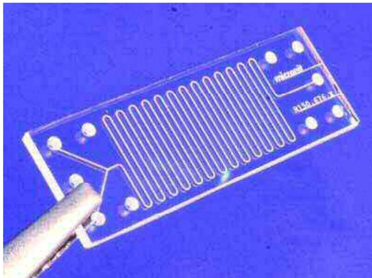
Glass Microreactor. The channels of the chip in the picture are 150 μm wide and 150 μm deep.
