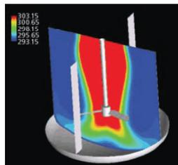
Heat distribution in a batch synthesis reactor
